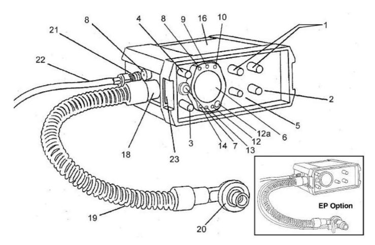
Figure 1a: Front view of ventiPAC showing accessories, features and the EP option
