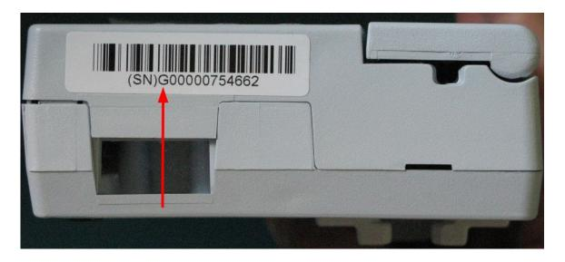
The 802.1b/g Wireless Battery Module (P/N 35162) is only compatible with pumps that include a 'G' preceding the serial number, as shown above. The 802.11b/g Wireless Battery Module (P/N 35162) should NOT be used with pumps that do not include a 'G' preceding the serial number.
