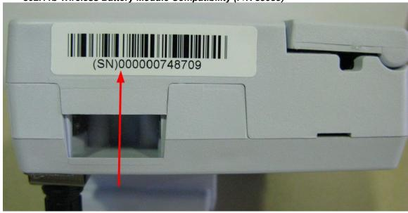
The 802.1b Wireless Battery Module (P/N 35083) is only compatible with pumps that DO NOT include a 'G' preceding the serial number, as shown above.
