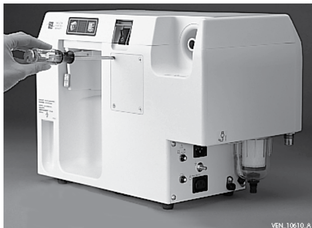
Figure 8-54. Replacing humidifier receptacle
