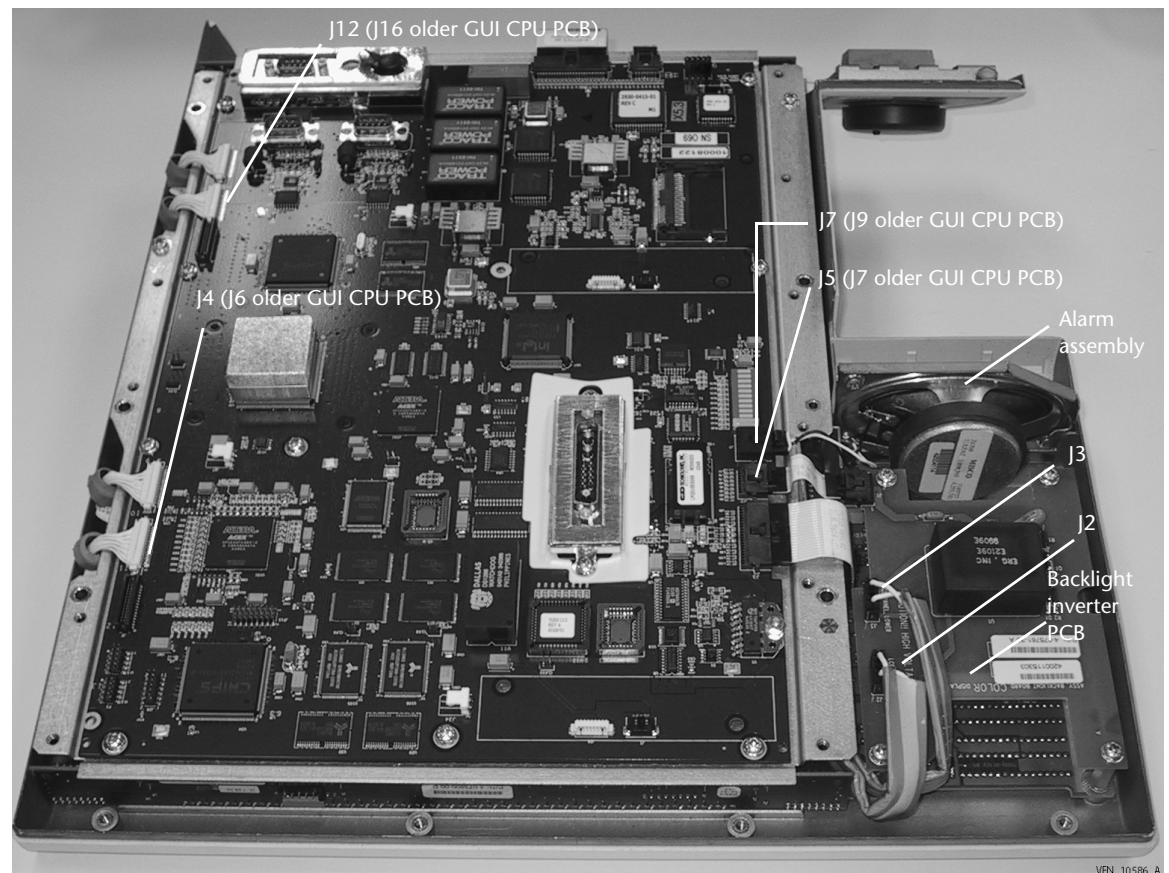
Figure 8-29. 9.4" GUI interior (TE GUI CPU PCB shown)
