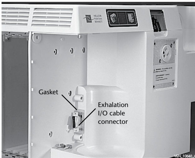
Figure 8-84. Removing BDU housing
