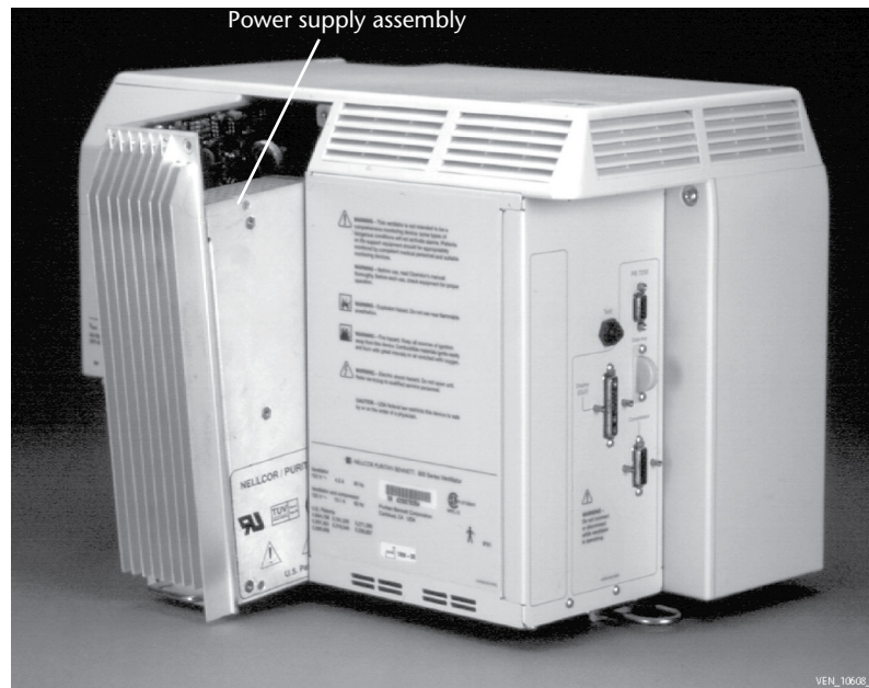
Figure 8-51. Replacing power supply assembly
