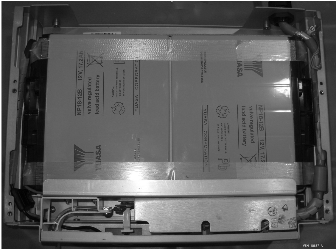
Figure 8-120. Four-hour battery cable routing
