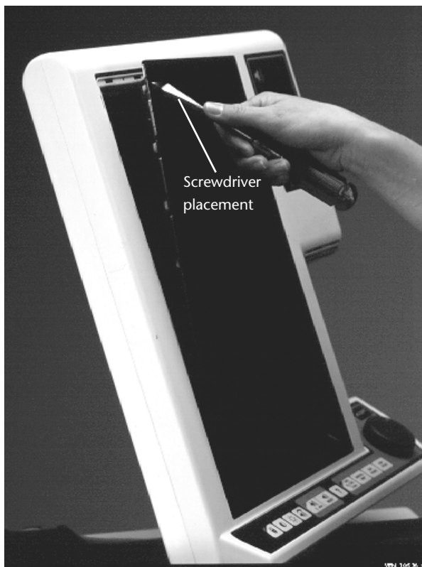
Figure 8-23. 9.4-inch touch screen bezel and window
