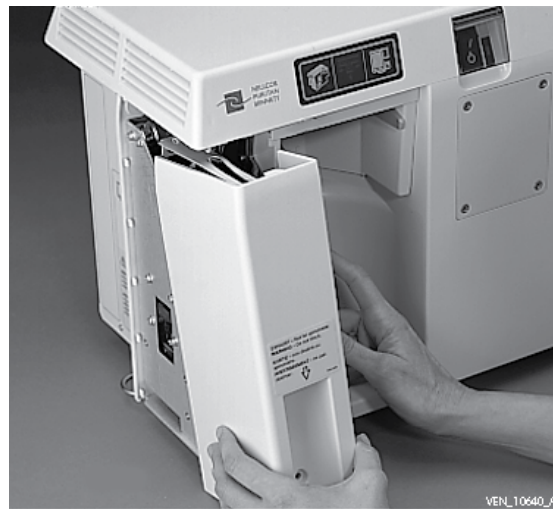
Figure 8-75. Removing exhalation module cover
