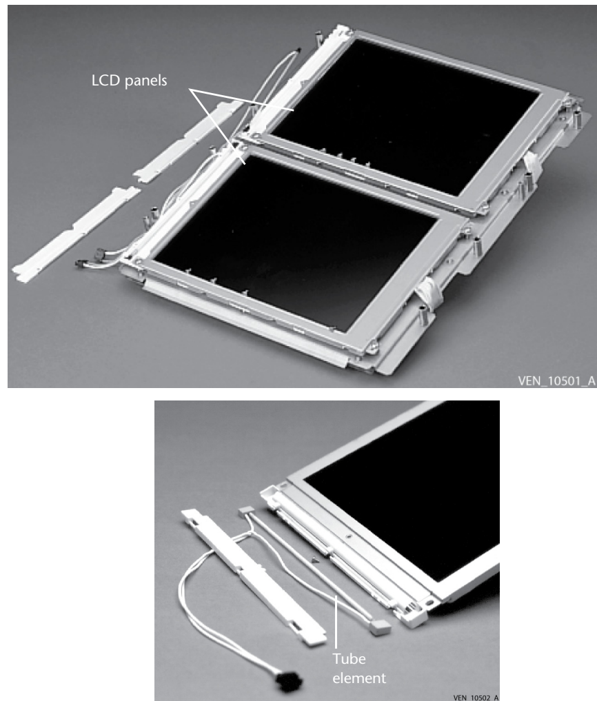
Figure 2-74. 9.4-inch LCD panels and backlight tubes
